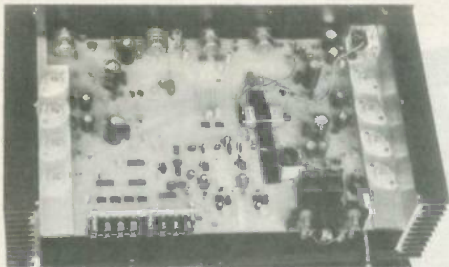
FIG. 10—MOST SWITCHES AND POTENTIOMETERS are soldered directly to the PC board; that eliminates much tedious wiring by hand.
