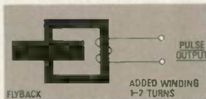
FIG. 5—USE THIS SCHEME to derive the flyback pulse required by the circuit in Fig. 4.
