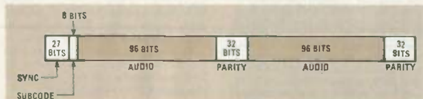
FIG. 1—MOST, BUT BY NO MEANS ALL, of the information in a frame of CD data is dedicated to the audio program.
